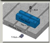
Installing the T-Slot Block is real fast and easy.The tabs on the T-Slot Block align to the machine table. Use bolt and T-Nut to attach T-Slot Block
